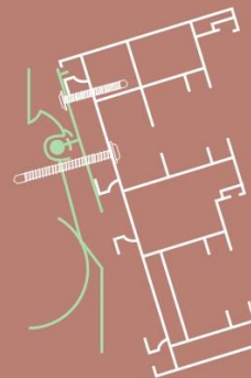
Screw from outside detail Frames can be screw-fitted through the coupler into the frame before the trim is added. This allows pre-glazed frames to be installed.
